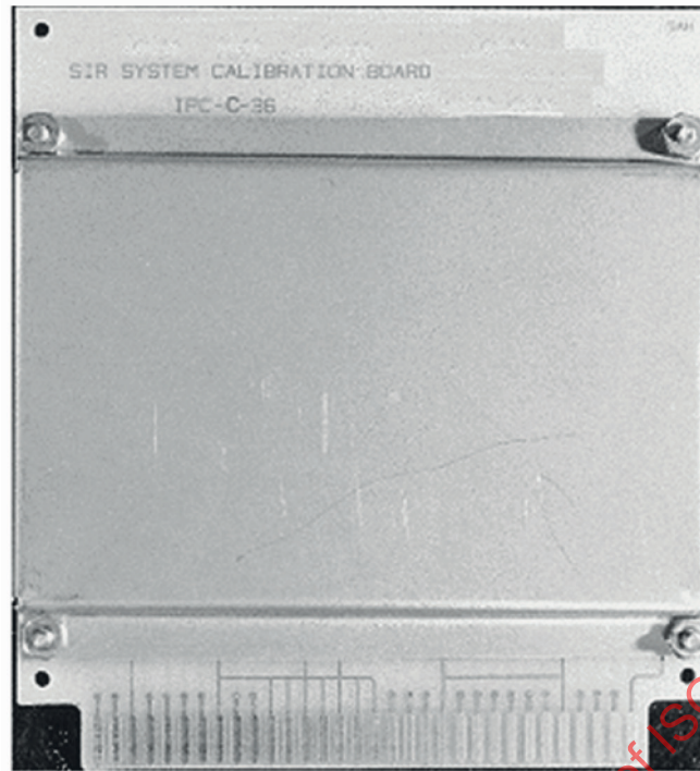
Figure 3 — Resistor verification board with protective cover
