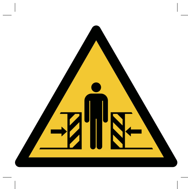
Figure A.5 — Example of warning sign: crushing hazard (ISO 7010 W019)
