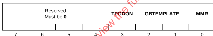
Figure 46 – Generic region segment flags field structure
