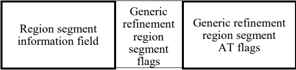
Figure 52 – Generic refinement region segment data header structure
