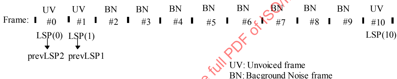
Figure 2.13 — Decoder parameter generation for background noise interval
