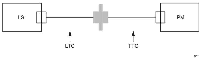
Figure 18 – Connection of LTC to TTC to verify attenuation of reference connectors
