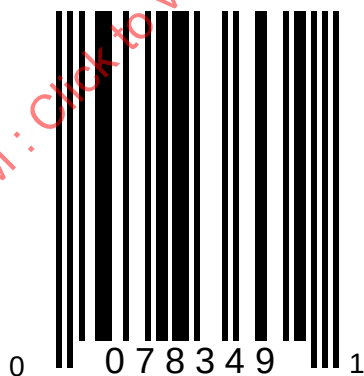
Figure 4: UPC-E bar code symbol (encoding “0 07834 00009 1” by zero suppression)
