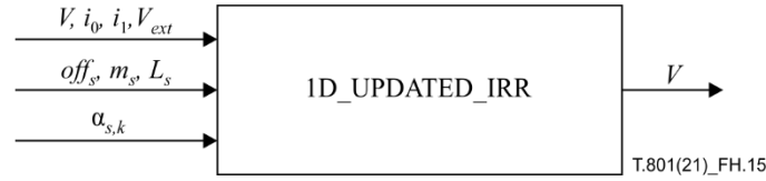
Figure H.15 – Parameters of the 1D_UPDATED_IRR procedure
