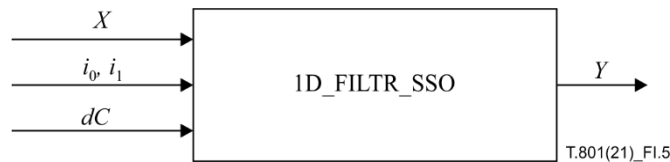
Figure I.5 – Parameters of the 1D_FILTR_SSO procedure
