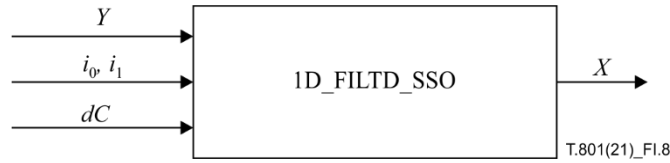
Figure I.8 – Parameters of the 1D_FILTD_SSO procedure
