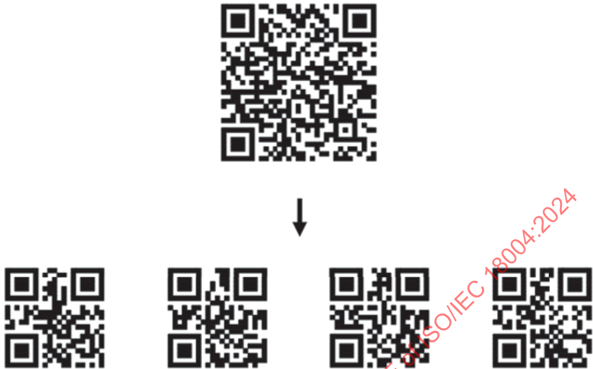
Figure 29 — Single symbol (above) and structured append series of symbols (below) encoding the text "ABCDEFGHIIJKLMNOPQRSTUVWXYZ 0123456789 ABCDEFGHIIJKLMNOPQRSTUVWXYZ"
