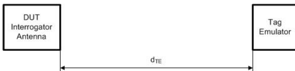
Figure 2 — Interrogator demodulation and turn around test setup
