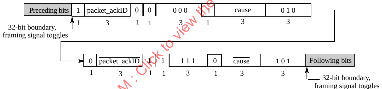
Figure 3-3. Type 2 Packet-Not-Accepted Control Symbol Format
