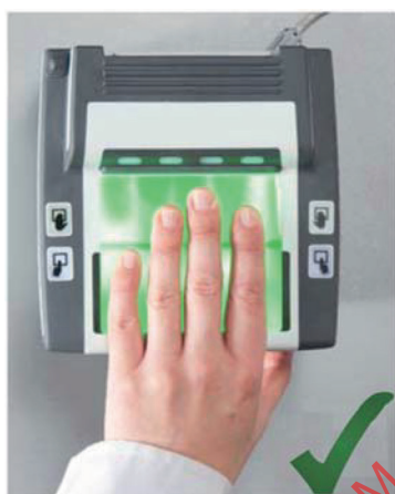
a) Prefer parallel fingers in relation to the edges
