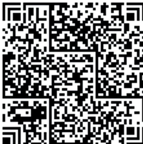
Figure K.22 — Masking result for Figure K.18 with masking pattern 11
