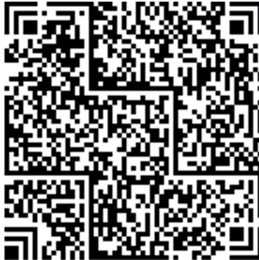
Figure K.20 — Masking result for Figure K.18 with masking pattern 01
