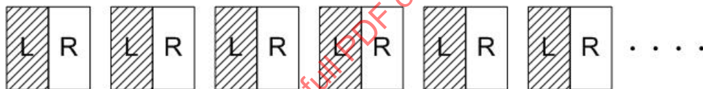
(a) Side-by-side (half) type stereoscopic sequence
