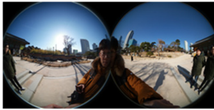
a) Example of a pair of circular input images prior to lens shading compensation
