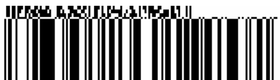
Figure 9 — A GS1 DataBar Expanded Composite symbol (with CC-A), encoding 01937123456789043103001234 and 911A2B3C4D5E respectively
