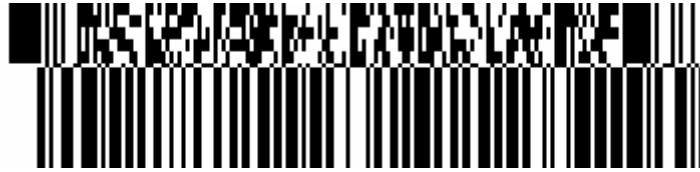
Figure 12 — A GS1-128 Composite symbol (with CC-C), encoding 00030123456789012340 and 02130123456789093724<FNC1>101234567ABCDEFG respectively
