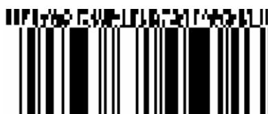
Figure 8 — A GS1 DataBar Omnidirectional Composite symbol (with CC-A), encoding 0103612345678904 and 11990102 respectively
