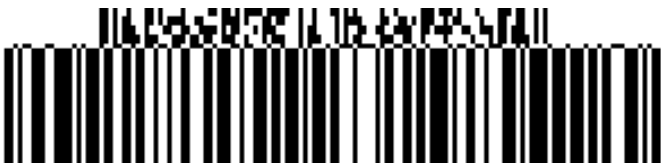
Figure 11 — A GS1-128 Composite symbol (with CC-A), encoding 0103212345678906 and 1A1B2C3D4E5F6G7H8 respectively
