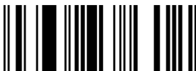
Figure 1 — GS1 DataBar Omnidirectional symbol representing (01)20012345678909
