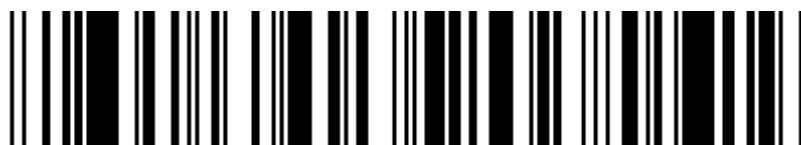
Figure 10 — GS1 DataBar Expanded symbol representing (01)98898765432106(3202)012345(15)991231
