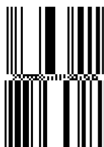
Figure 6 — GS1 DataBar Stacked Omnidirectional symbol representing (01)00034567890125
