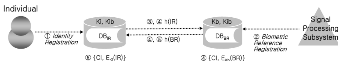
Figure A.1 — Secure binding between separated DB_{IR} and DB_{BR} (Case A)
