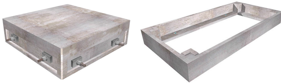
Figure A.4 — Foundations in industrial construction
