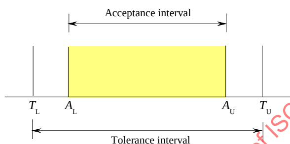
Figure 1 – Binary conformity assessment where decisions are based on measured quantity values. The true value of a measurable property (the measurand) of an item is specified to lie in a tolerance interval defined by limits ( T_L, T_U ). The item is accepted as conforming if the measured value of the property lies in an interval defined by acceptance limits (see 3.3.8) ( A_L, A_U ), and rejected as non-conforming otherwise.
