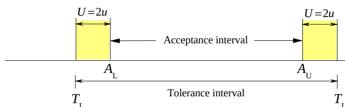
Figure 10 – Two-sided acceptance interval created by reducing the tolerance interval on either side by the k = 2 expanded uncertainty U = 2u . This is the default decision rule established in ISO 14253-1 [21].
