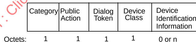
Figure 8-460i—GDD Enablement Request frame Action field format
