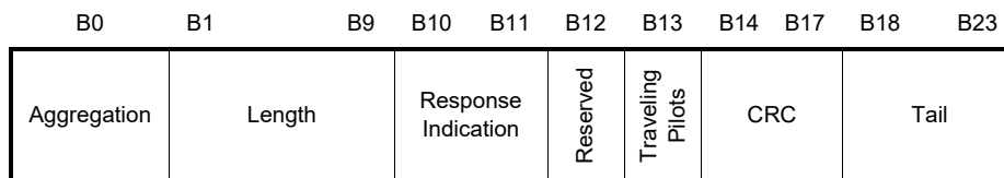
Figure 23-12—SIG-A2 structure for SU PPDU
