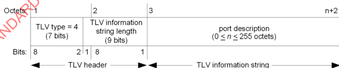
Figure 8-7—Port Description TLV format
