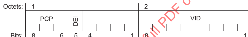
Figure 9-1—VLAN TCI format
