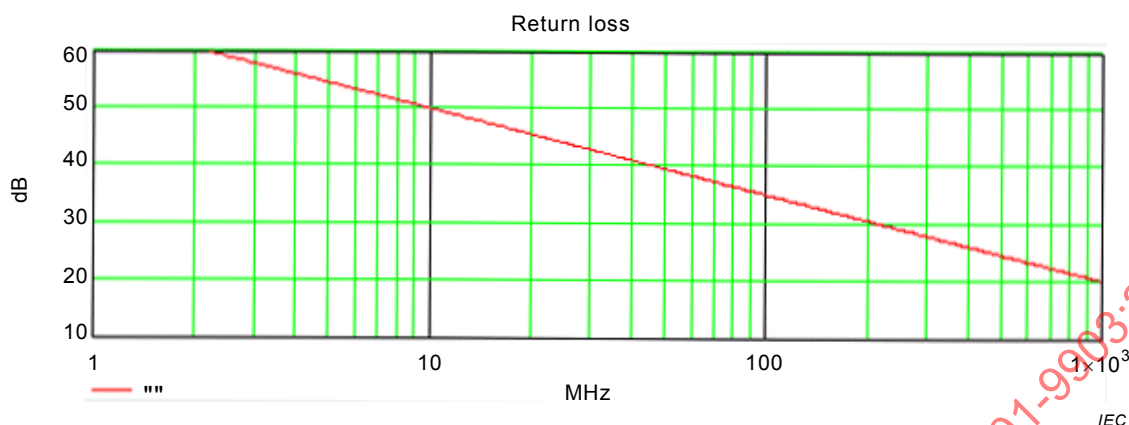
Figure 11 – 100 m cable return loss without reflection at both ends
