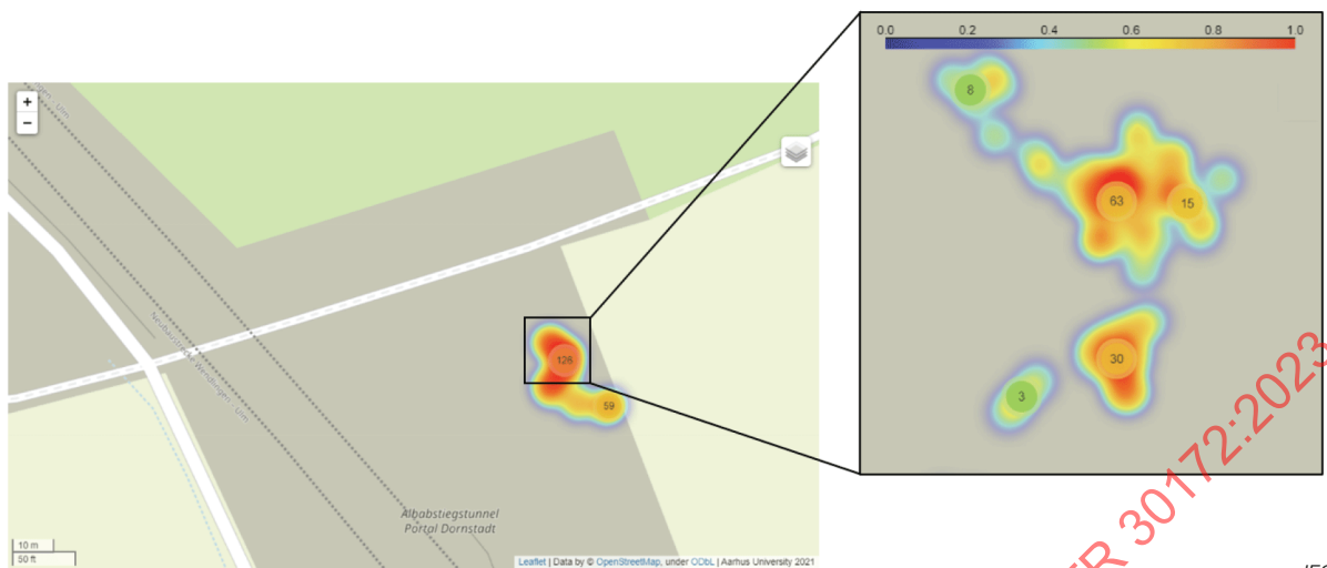
Figure B.2 – Identification of close proximity events between heavy machinery
