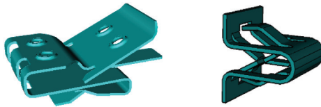
Figure 37 — Clips sliding onto a flat surface
