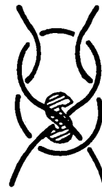
FIG. 4 – Weaver's knot – S-type
