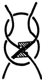
FIG. 3 – Weaver's knot – Z-type
