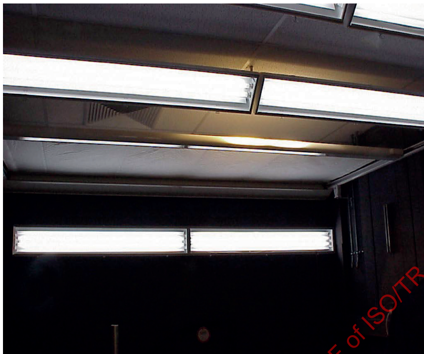
Figure 12 — Sailcloth pulled across fully for indirect illumination / scattered light (see number 5 in Figure 11 )
