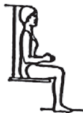
Figure G.1 — Illustration of the seated height (SEATHT), as defined in the MCW test reports
