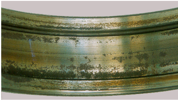
Figure 22 — Corrosion on roller bearing outer ring
