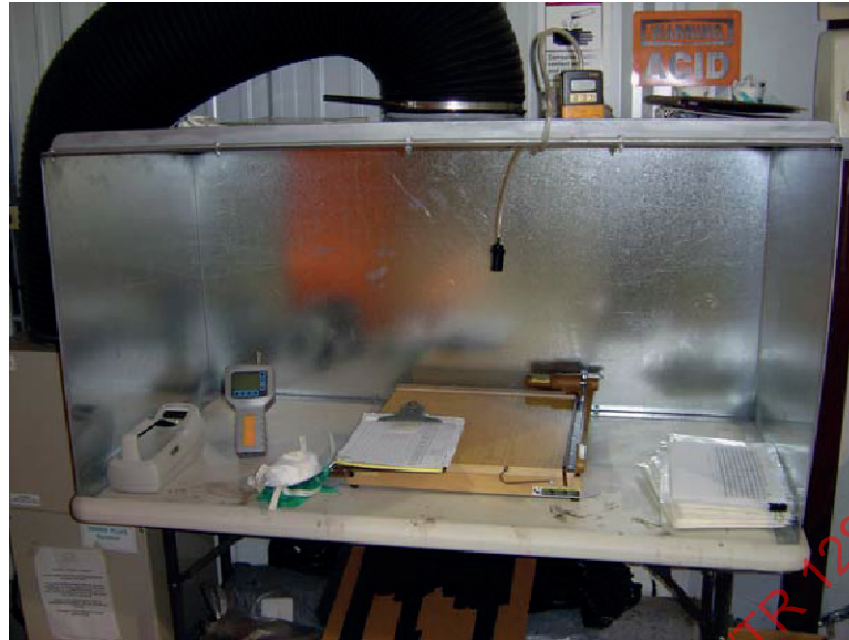
Figure 7 — Enclosing hood with HEPA exhaust (from NIOSH Progress Toward Safe Nanotechnology in the Workplace [278] )
