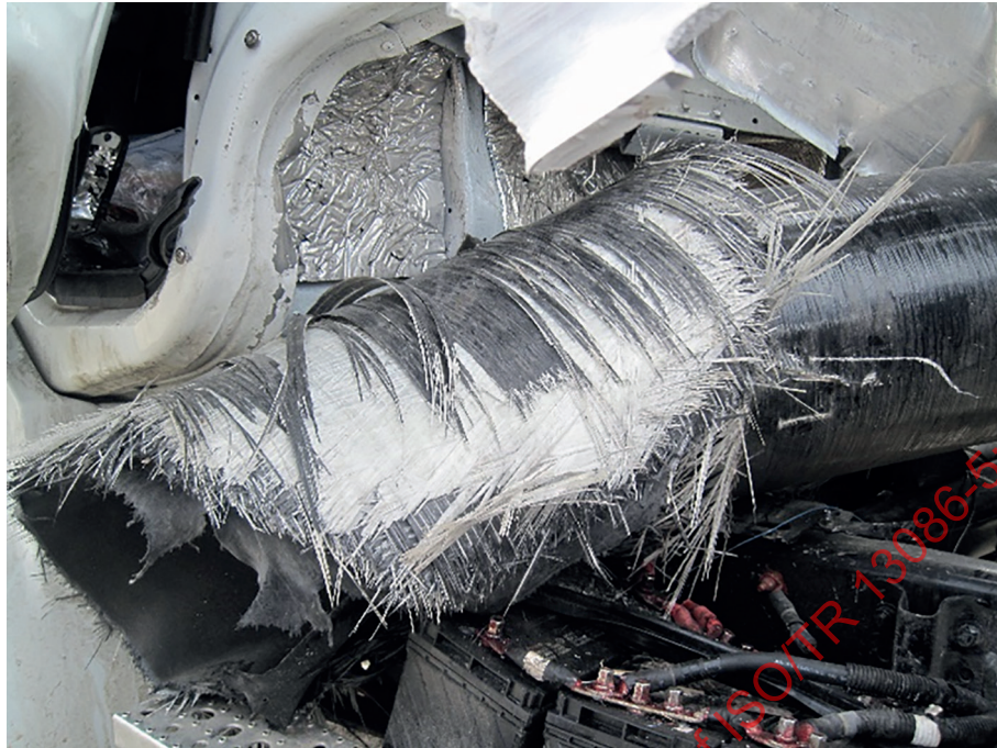
Figure 8 — Fuel container ruptured by impact
