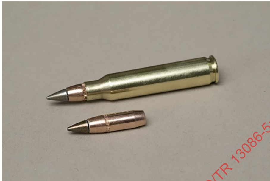
Figure 3 — Cartridge and bullet for high velocity impact (gunfire) test
