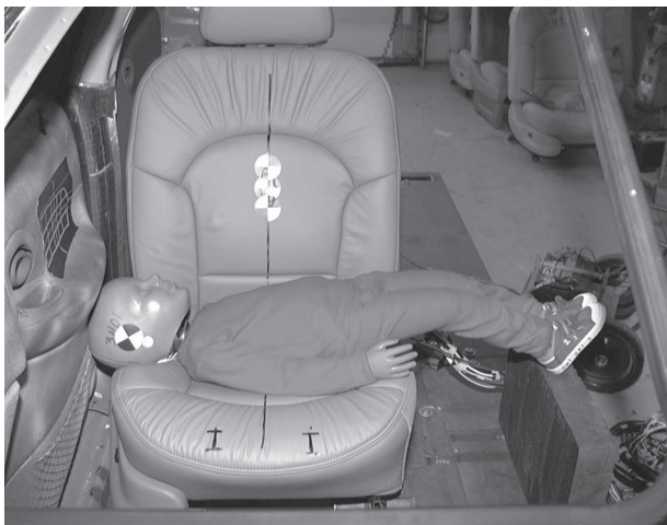
Figure 8 — Child lying across seat with head against the door trim panel (door/quarter-mounted air bag system)
