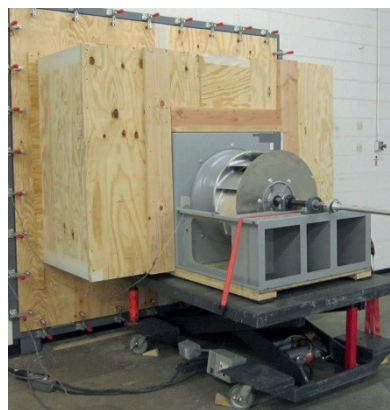
Figure 18 — Inlet pillow block bearing with support
