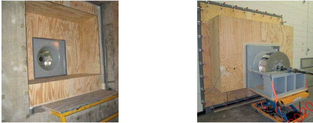
Figure 20 — Inlet cabinet with side wall spacings 1D right, 1D top and 1D left
