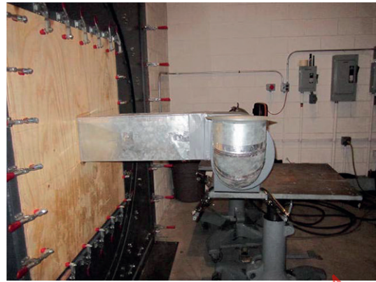
Figure 23 — Views of the FC centrifugal fan with the inlet elbow at 12 o'clock
