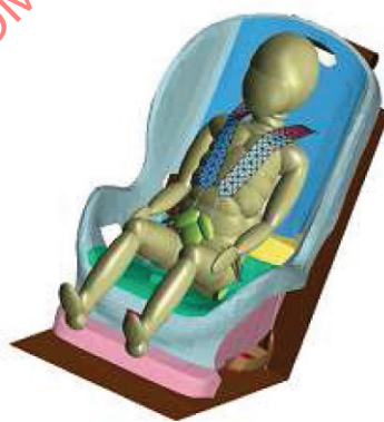
Figure A.2 — CAE model of child restraint example[33]
