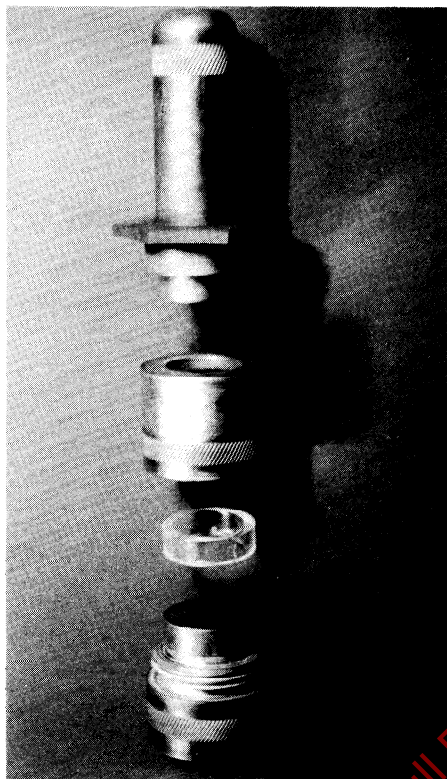
Figure A.2 — Apparatus for making powder tablets
