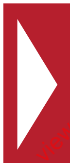
Figure 3 — Example of directional indicator for fire equipment
