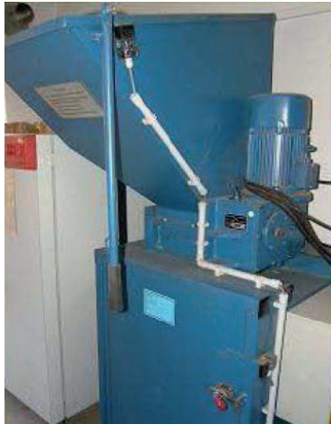
a) Retsch cutting mill, particle size 5 mm to 10 mm
