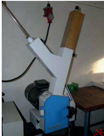
b) Retsch cutting mill 2 000, particle size ~ 1 mm
