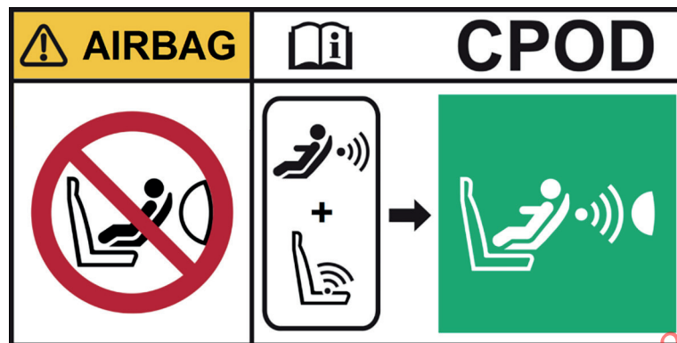
Figure A.2 — Labelling of CPOD vehicles
