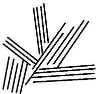
Figure 3 — Example sketch of turbostratic few-layer graphene particle
