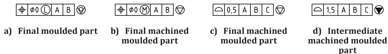
Figure 12 — Examples of geometrical tolerances with datum references
