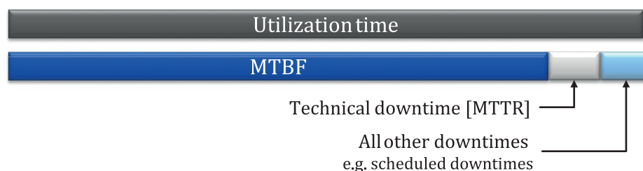
Figure 3 — MTBF as a component of utilization time
