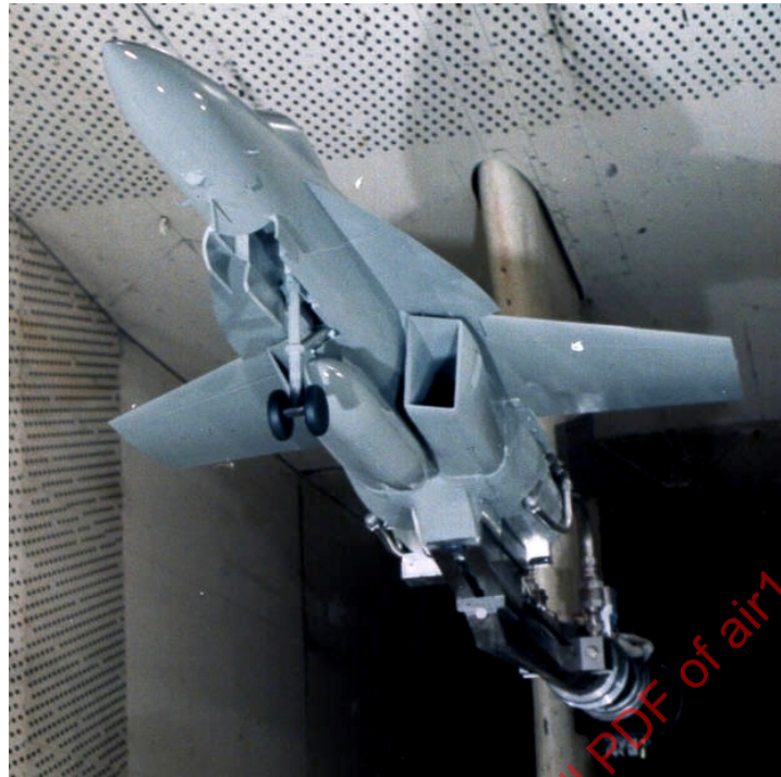
FIGURE 99 - 0.176-SCALE F-18E/F MODEL USED FOR INLET VERIFICATION TESTS
