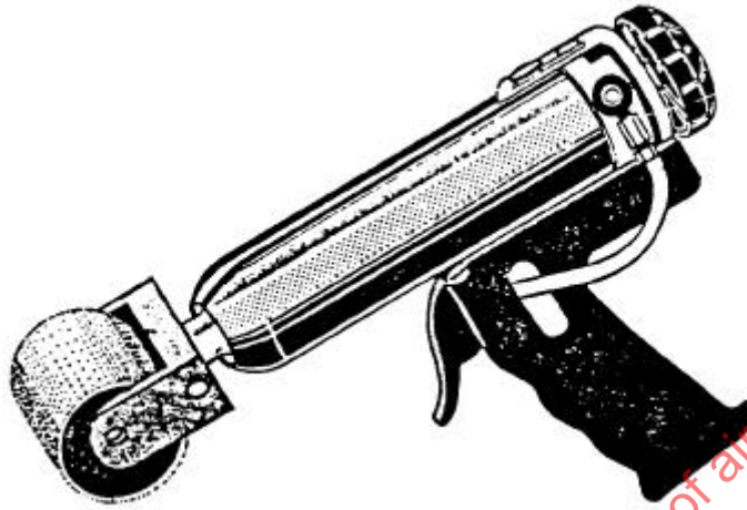
FIGURE 32 - Roller Nozzle for Faying-Surface Sealing Application
