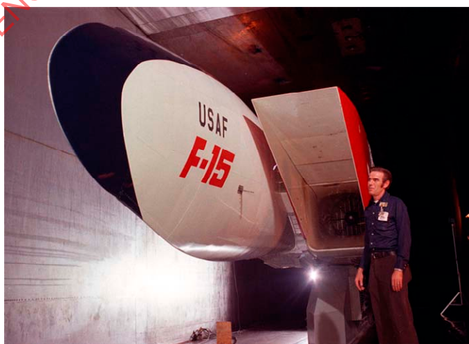
FIGURE 59 - FULL-SCALE F-15 INLET WITH MODIFIED FOREBODY
