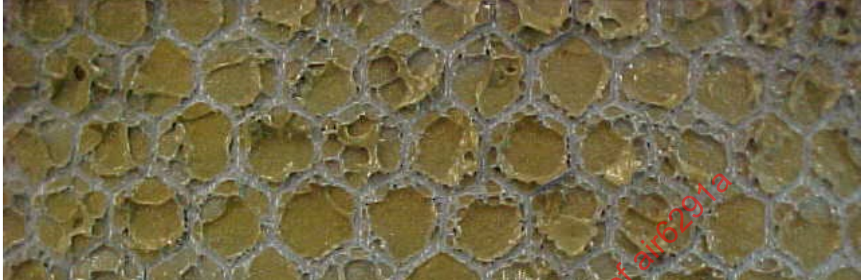
Figure 10 - Foaming of adhesive due to the improper application of vacuum pressure
