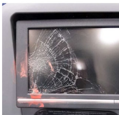
Figure B1 - Collins Aerospace HIC test post-test photos - modified monitors (Zones C and A)
