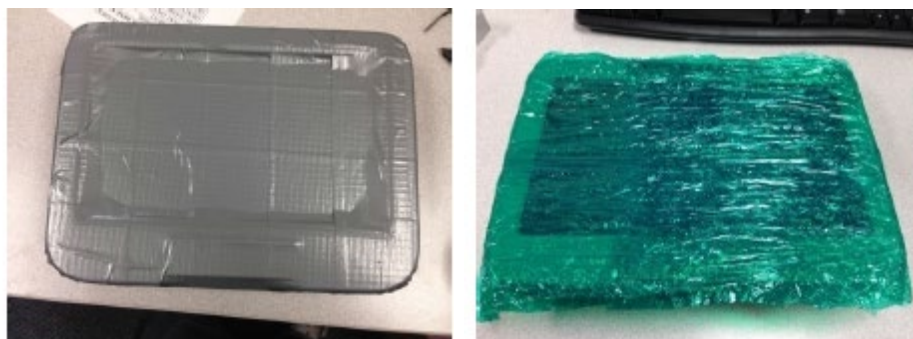
Figure 16 - Panasonic 10.6-inch monitor with duct tape and mover's wrap added
