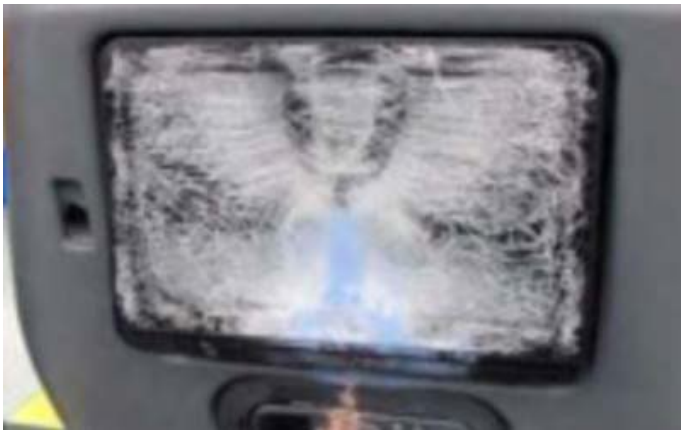
Figure B2 - Recaro HIC test post-test photos - baseline and modified monitor
