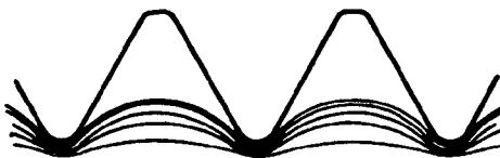
Figure 3 Flow Lines - Rolled Thread
